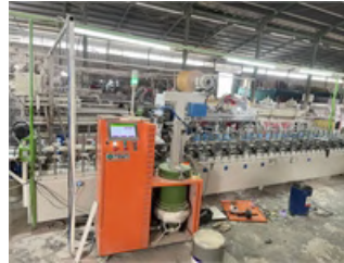
WPC MACHINE to produce Wood-Plastic Composite
