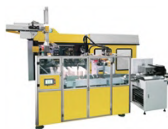
CUTLERY PACKING AUTOMATION Function: 1. Take out products from the mold 2. Accumulation of parts in stack. 3. Adjustable numbers of parts on the stack. 4. Packaging with wrapping paper
