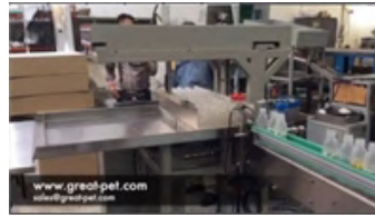
BOTTLE PACKING MODEL: BTB-01 Automatic bottle packaging machine of Maha Thani Helps to reduce a lot of staff use because customers have trouble storing bottles that come out each minute. The company has therefore developed an automated storage system for 6,000 bottles per hour, reducing 5 people in the bottle packaging process.
