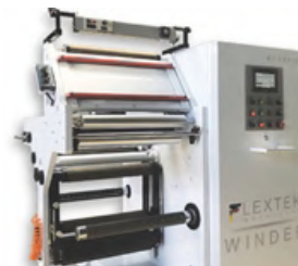
R1 WINDER - DOCTOR REWINDER R1 is a medium sized doctor revider allowing to re-work finished rolls and eliminating errors in rolled materials at high speed. Developed to focus on efficiency, decreasing waste and increasing companies productivity. Additional rewinding performed on this machine has a purpose to correct quality of material web, control of print quality, extract of faulty material, and if required to cut off edges.
