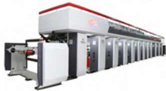
ELECTRONIC LINE SHAFT ROTOGRAVURE PRINTING MACHINE printing speed : 300-450M/MIN;Disc type Unwinder&Rewinder
